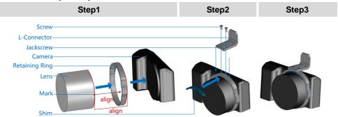
**Step1:** Put retaining ring through lens before mounting onto camera, accurate the alignment by matching the mark.
