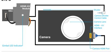
Step1: Connect the gimbal HDMI-AV module to camera HDMI port with a HDMI-AV connection cable.
